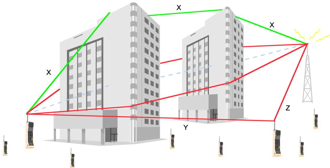
It can be appreciated from Fig 1 that the signal loss can vary tremendously based on the choice of path. Consider that path X represents a mobile to base station route. By choosing instead to hop through the LOS paths Y & Z one could easily imagine a 30dB loss reduction i.e. for the same data throughput the total TX power at each hop could be reduced by a factor of 1000 e.g. 1mW instead of 1W.
